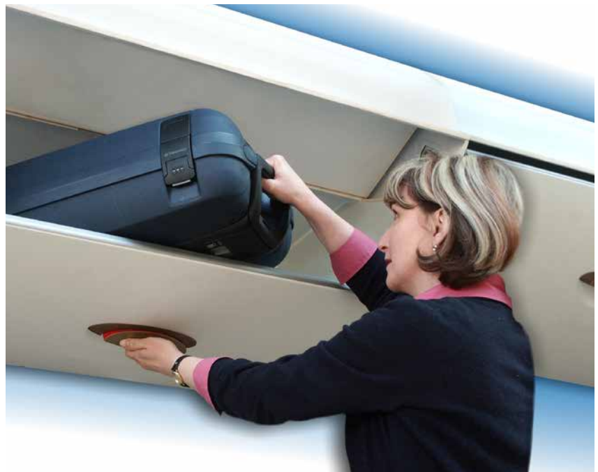
Full automatic stowage BIN actuation with lock / unlock and flight attendant feedback
