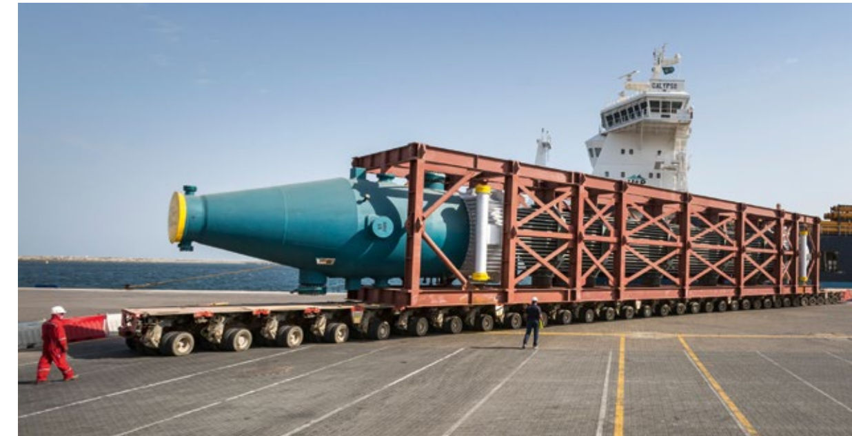
SCHMIDT'SCHE® Syngas Cooler at the port on its way to the plant construction site
