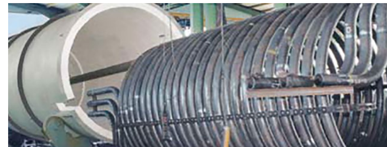
SCHACK® Fired Heater internals
